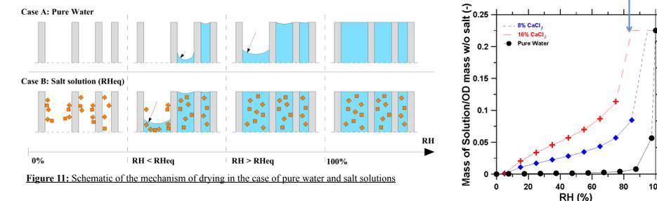
Figure 12: Desorption curves for ceramic samples saturated in CaCl<sub>2</sub> solutions and pure water
