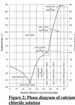
Figure 2: Phase diagram of calcium chloride solution
