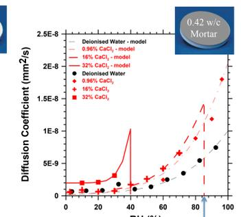
Figure 10: Diffusion coefficient for CaCl<sub>2</sub> solutions and pure water measured on mortar sample
