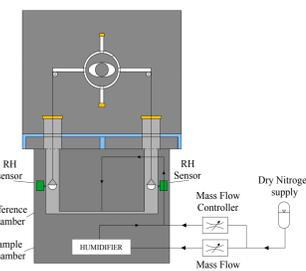
Figure 4: Du Noüy Ring tensiometer (Pease et al. 2005)
