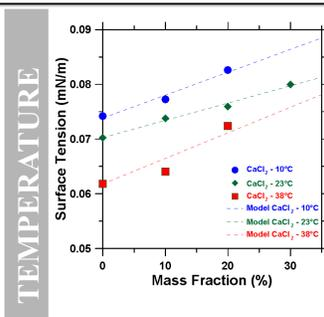
Figure 8: Surface Tension of deicing salts as function of temperature
