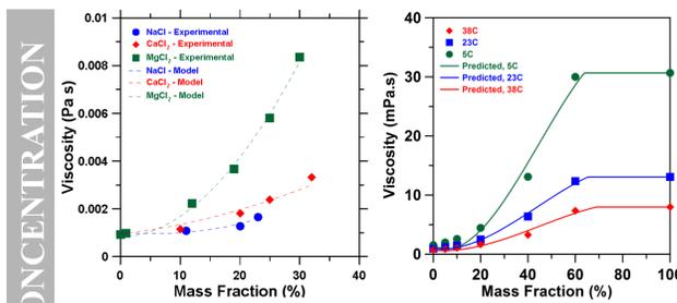
Figure 5: Viscosity as function of concentration for a) deicing salt solutions and b) SRA solution
