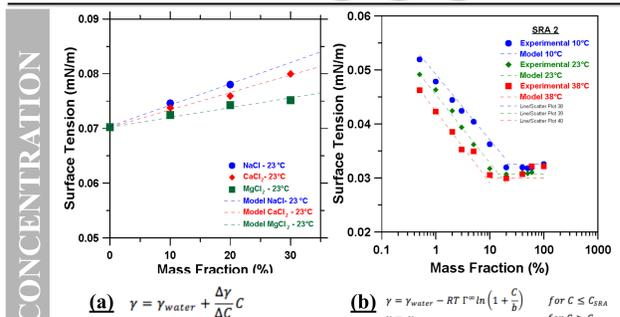
Figure 7: Surface tension as function of concentration for a) deicing salt solutions and b) SRA solution
