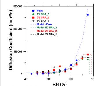
Figure 13: Diffusion coefficient for mortar samples saturated in water-SRA solutions
