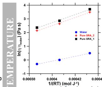
Figure 6: Viscosity as function of temperature for SRA solution
