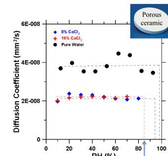
Figure 9: Diffusion coefficient for CaCl<sub>2</sub> solutions and pure water measured on porous ceramic
